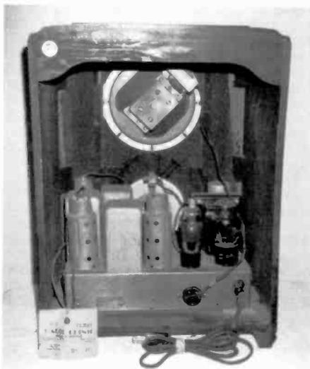
Figure 2. The condition of the converted chassis equals that of the cabinet. The added Type 5Y3 rectifier tube is located on the far right of the chassis.
