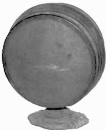
**RCA RADIOLA 100** – This drum speaker was manufactured by the Radio Corp. of America to accompany its Radiola 20 and Radiola 25 radios. (Clark Trissell – Lincoln, NB)
