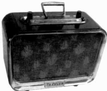
**TRAV-LER MODEL TR-262** – This early battery-powered transistor portable radio has six plug-in transistors. It is unique in that it has the same appearance from front or back, and the dual, slide-rule dial can be read from either side. This model was also branded and sold by Hallicrafters. (Ray Chase – Plainfield, NJ)
