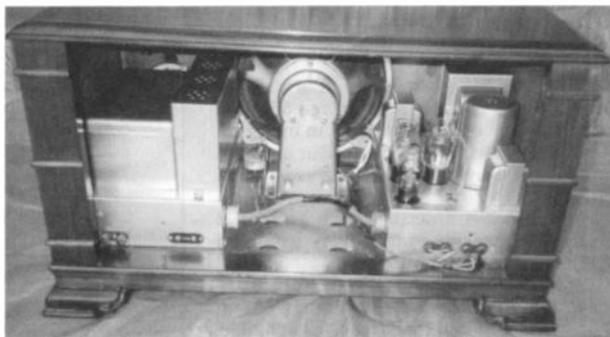
Figure 2. Rear view shown open to expose the two chassis: the 4-tube tuner is at the left, and the 4-tube power supply/amplifier is at the right.
