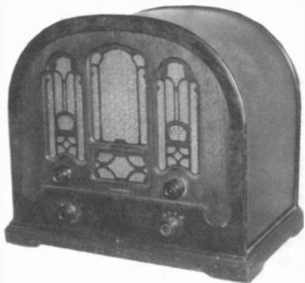
**ATWATER KENT MODEL 708** – This 8-tube cathedral was manufactured in 1933 by the Atwater Kent Manufacturing Co. of Philadelphia, Pennsylvania. It measures 12½" high and 16" wide. The dial appears behind a small window opening at the top. (*Wally Worth – Wollaston, MA*)
