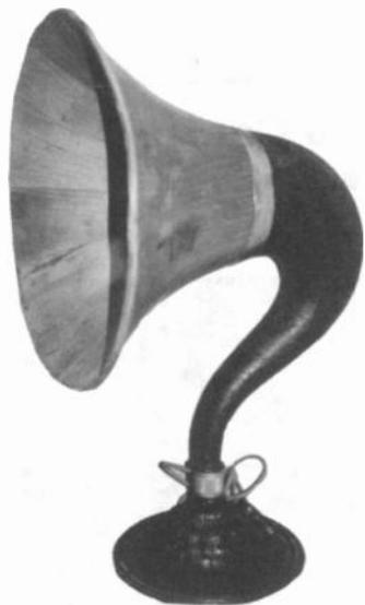
**MUSIC MASTER HORN SPEAKER** – This horn speaker was manufactured by the General Radio Co. of Cambridge, Mass. It has the hard-to-find spruce, wooden bell with a 13 $\frac{3}{4}$ " diameter, and it stands 22 $\frac{1}{4}$ " tall. (*Wally Worth – Wollaston, MA*)
