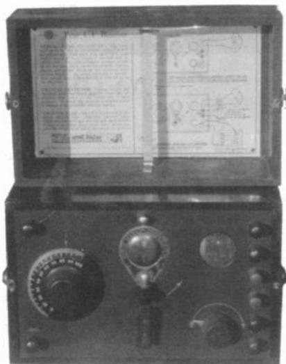
**HOME TYPE CT RECEIVER** – This unique receiver was sold in 1922 by the Home Radio Corp. at 100 Madison Avenue in New York City. The operator could either use the catwhisker crystal detector viewed behind a glassed-in dome (above center), or flip the center bottom switch to the one internal tube for detection. (*Merrill Bancroft – Townsend, MA*)
