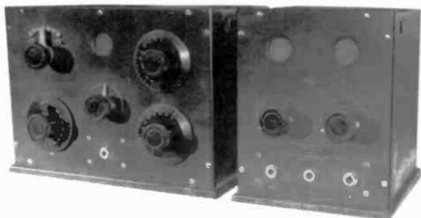
**CARDWELL RECEIVER AND AMPLIFIER** – This combination of 1-tube receiver and 2-tube amplifier was manufactured by the Allen D. Cardwell Mfg. Co. of Brooklyn, New York. While the audio amplifier is identified as Type 103-A, the receiver has no model number. (Merrill Bancroft – Townsend, MA)
