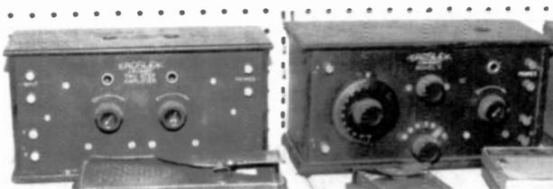
This Crosley 2-tube amplifier (left), and 1-tube receiver, (right), have over-hanging lids with holes to accommodate tipped and oversized tubes. These features indicate their early production. The pair brought a bid of \$750.
