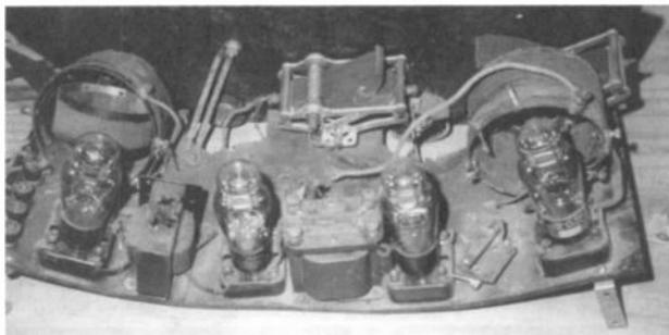
Figure 2. View showing how badly the chassis had deteriorated over the years.
