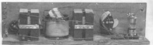
Figure 2. A component view of a capacitive feedback radio.
