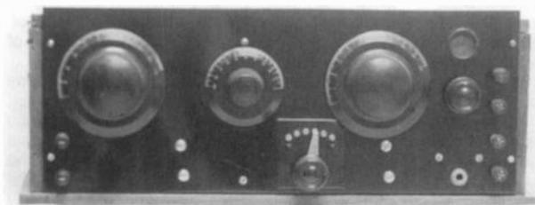
Figure 3. The panel of an inductive feedback radio.
