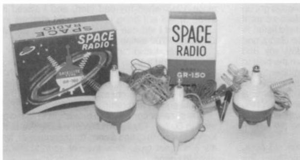
**SATELLITE GR-150 & GR-160 TOY RADIOS** – These "space radios," made in Japan in the 1960s, are germanium crystal sets that came with ear-plug phones. I have three types, in red, blue, and green. (Erwin Macho – Vienna, Austria)
