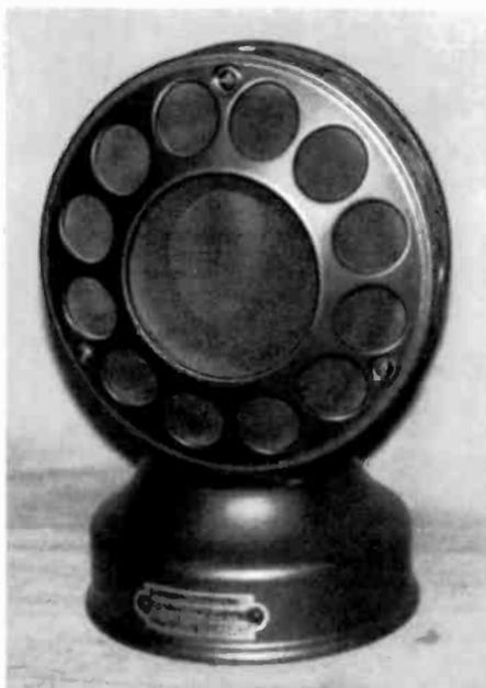
Figure 9. The Kodel "Microphone" speaker.
