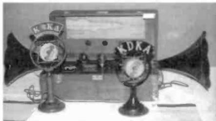
In the contest was this rare collection of radio station KDKA microphones and a Western Electric amplifier having two horns attached.
