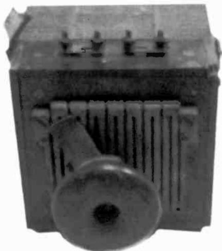
**PHANTOM LOAD** – This dummy load was manufactured in 1910 by the States Company of Connecticut. It has a finger-jointed oak case six inches square. It is very heavy. (Paul Recuperero – Portsmouth, RI)
