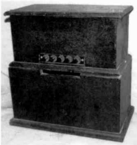
Figure 5. The rear of the Kodol Model C-14 with battery box below.
