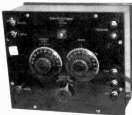
**NORTHERN ELECTRIC MODEL R1** – Patented in 1923, this 1-tube receiver was manufactured by the Northern Electric Company, Ltd. It uses a single Type 215A tube that protrudes through the heavy Bakelite panel. The wooden cabinet is quite similar to that of the Western Electric 7A amplifier. (*Wally Worth – Wollaston, MA*)
