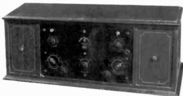
**RCA REGENOFLEX** – The RCA Regenoflex, introduced in 1924, employs a tuned RF amp, a regenerative detector, and two audio stages with four WD-11 tubes. The antenna input variometer is labeled "Volume," and the variable regeneration control is labeled "Amplification." With two other tuning controls and the filament rheostat, operation would be a handful for a novice. This set is seldom seen. Two side compartments provide space for the required batteries. (Ray Chase – Plainfield, NJ)
