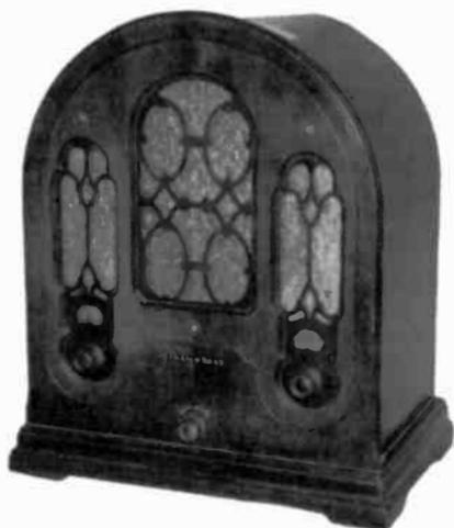
**ATWATER KENT MODEL 165** – This 1933 cathedral operates with a 5-tube superhet chassis. It was one of the less expensive cathedrals sold by Atwater Kent. (Wally Worth – Wollaston, MA)
