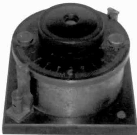
**TUNING CAPACITOR, MANUFACTURER UNKNOWN** – This variable air capacitor measures  $4\frac{1}{2}$ " x  $3\frac{1}{2}$ ". It has 50 aluminum plates that are  $3\frac{3}{4}$ " round. The Bakelite dial sits on a brass case with a Bakelite base. (Paul Recupero – Portsmouth, RI)
