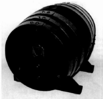
*Figure 1. Radiokeg Model RK-S-5 recently restored using a diode as a replacement for a resistance line cord.*
