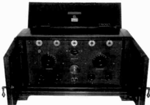
**GECOPHONE BC2050** – This 1924 5-tube battery set was the company's top-of-the-line receiver. It is considered rare, as most British radios of the early 1920s were 2- or 3-tube sets. All British radio manufacturers had to pay a rather high royalty to Marconi for each tube in the circuit. (Jim Taylor – Boumemouth, England)
