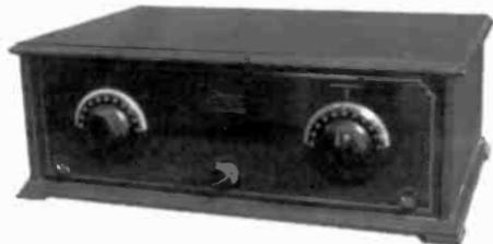
**SILVER-MARSHALL TYPE 630** – This 1928 “Shielded Six” uses five Type 201 tubes, plus a Type 112, has four tuned stages, three of which are in separate shielded compartments. It was advertised as an AC set when used with a companion battery eliminator. (Ray Chase – Plainfield, NJ)
