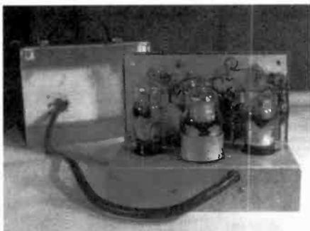
Figure 4. The Model T-22 receiver with its rear cover removed, showing the tube lineup.
