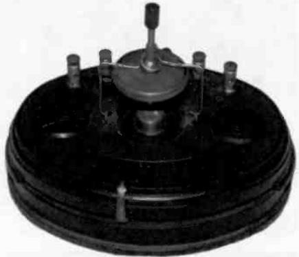
**MARCONIPHONE "BABY"** – This crystal set was manufactured by the Marconi Co., Ltd., of Great Britain. The crystal element is enclosed in glass. Tuning is accomplished by sliding the small arrow-dial around a slot in its Bakelite base. (*Jim Taylor – Bournemouth, England*)
