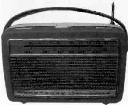
**NORDMENDE STRADELLA** – This 1962, 6-transistor, AM/FM radio was made in Germany. Its all-wood case is covered with a grained leatherette. It has a telescoping antenna and the power cable terminals clip on to a 6-volt battery. (*Francis H. Yonker – State College, PA*)
