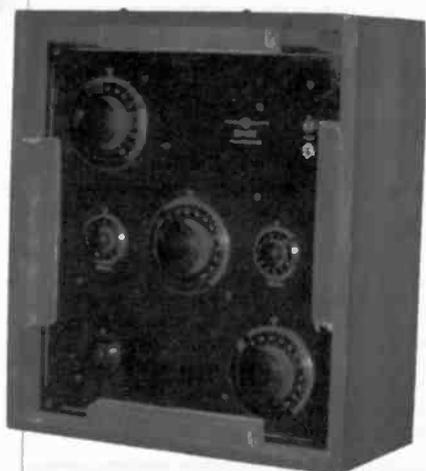
**FADA TYPE 196-A** – This 5-tube, Neutrodyne receiver was purchased in its original packing crate. It was sold in 1924 as a panel set for installation only in some of the Victor phonograph cabinets. The original owner operated it as he had purchased it — he never took it out of the wooden packing case! (Joseph G. Jackson – Macon, GA)
