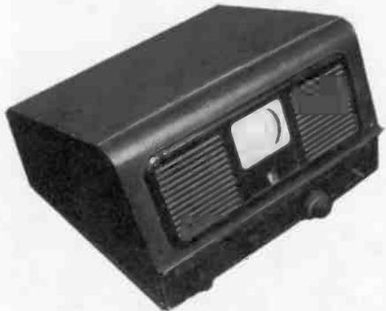
**PILOT MODEL TV-37** – This 1949 television set, with synchronous tuning, was the first TV to sell below \$100. Its price was just \$99. The picture tube is only 3" in diameter (3KP4). (*Dave Crocker – Mashpee, MA*)
