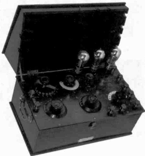
**RADIO INDUSTRIES TYPE 3VA** – Manufactured in 1922 by Radio Industries, Ltd., this 3-tube (valve) receiver has World War I type construction. (Jim Taylor – Bournemouth, England)
