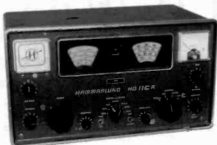
**HAMMARLUND MODEL HQ-110A** – This metal-cased radio is a quality shortwave receiver. It tunes from 160 to 6 meters. The circuit uses the following tubes: (2) 6BZ6, 6BE6, 12AX7, 63A6, 6AZ8, 6BJ7, 6AQ5, 6C4, 5U4, and 0B2 regulator. (Clark Trissell – Lincoln, NB)
