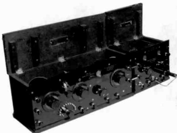
**KENNEDY TYPE 281 AND TYPE 521** – This 2-unit combination set is made up of a Kennedy Type 281 1-tube receiver and a Type 521 2-tube amplifier. The set was manufactured in 1921 by the Colin B. Kennedy Co. of St. Louis and San Francisco. The receiver has regenerative circuitry and tunes from 180 to 620 meters. (Dave Crocker – Mash-pee, MA)
