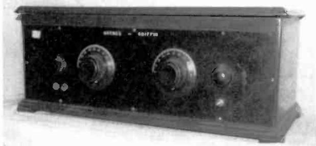
*Figure 1. This front panel view of the Haynes-Griffin Superhet shows the two main tuning control dials, the two rheostat controls beside the two dials, the off-on switch (lower right), and the two phone jacks at the far left.*
