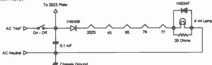
The on/off switch must be rewired to switch the hot side of the AC line. Also, the correct polarity of the 1N5347 zener diode is also shown in the revised schematic.
