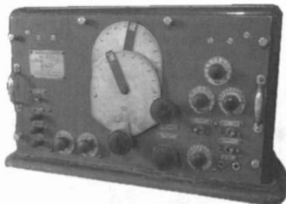
**RCA MODEL AR-60-5** – This “commercial grade” receiver was built around 1935; however, the knobs look much older. It uses the following eleven tubes: (4) 6D6, (2) 6C6, (1) 6B7, (1) 6F7, (1) 41, (1) 84, and (1) 991. Weighing about 95 pounds, it receives from 1500 Kc to 25 MHz and can operate on 110, 220, or 6 volts. It also has a bullet-shaped external speaker (not shown). (*Zach Taylor – Lincoln, IL*)
