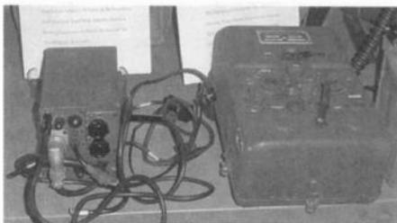
The rare Eureka beacon set used during World War II. The gear operates in the UHF band between the 214 to 234 Mc range.
