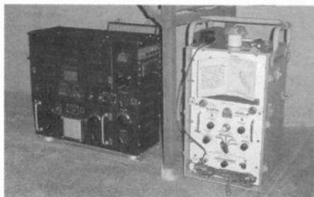
At left is a BC-375 aircraft transmitter from World War II. At right is an RMCA ET-8053 lifeboat transmitter, also known as AN/SRC-6. The transmitter and receiver, ca. 1953, operate on 500 Kc and 8364 Kc CW. These were the MF (Medium Frequency) and HF (High Frequency) maritime emergency frequencies. Crank handles fit into the sides of the radio and are hand-rotated for power.
