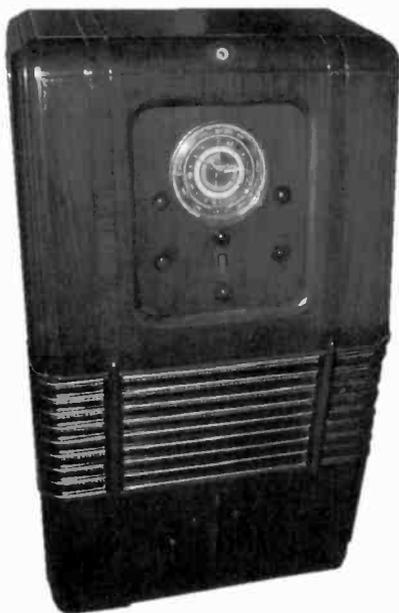
Figure 9. Sparton of Canada offered a 15-tube set also housed in an unusual cabinet. It covered the BC, SW and weather bands.
