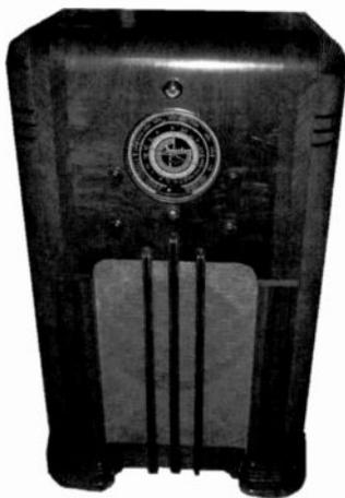
*Figure 3. Sparton produced a number of console models. This Model 867 is an 8-tube console with a rated audio output of 7 watts. It tuned the broadcast and SW bands.*
