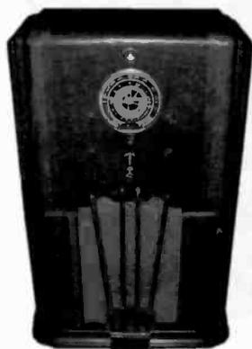
Figure 4. The Model 987, a 9-tube console in a walnut cabinet has a 6-inch silver mirror dial and tunes 535 kHz to 19.5 MHz.
