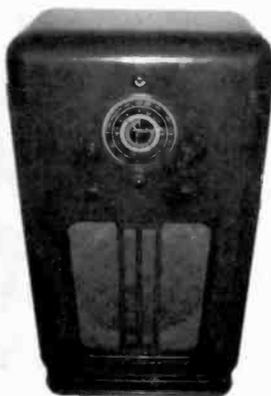
Figure 5. The Model 1167, an 11-tube set, is similar in appearance to the Model 867. In addition to the broadcast and SW bands, the radio also tunes the 140-420 kHz weather band.
