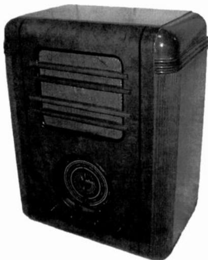
*Figure 2. Housed in an Art Deco cabinet, the Sparton Model 617, a 6-tube table radio from 1937, featured Sparton's photochromatic dial.*
