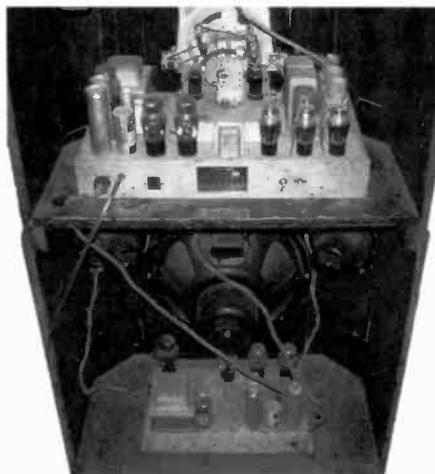
Figure 8. Sparton's top-of-the-line set, the Model 1867, used two chassis. This rear view shows the tuner chassis on top and the audio output/power supply at the bottom. A 15-inch speaker and two angle-mounted tweeters result in high quality sound.
