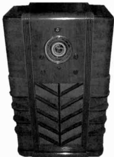
Figure 7. The Model 1867 Triolean, an 18-tube set, is housed in a striking cabinet. Its SW coverage extends to 60 MHz.
