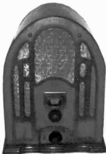
**UNIVERSAL MODEL 42** – This cathedral was manufactured by the Universal Radio & Television Corp. It has a 4-tube TRF chassis using (2) Type 24s for RF amps, (1) Type 47 for audio and (1) Type 80 as a rectifier. It sold for \$160 in 1932. (Jerry Wieland – Hoffman Estates, IL)
