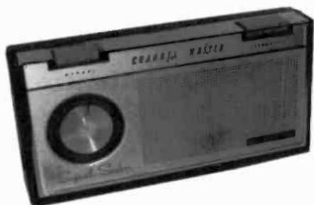
**CHANNEL MASTER MODEL 6459** – This 10 transistor portable was manufactured in the late 1950's or early 1960's. It was marketed as the "Signal Seeker" which featured a motor in the rear that automatically tuned the stations by depressing the right-hand button. The left-hand button is for tuning manually. (Gerald Silver – Tamarac, FL)
