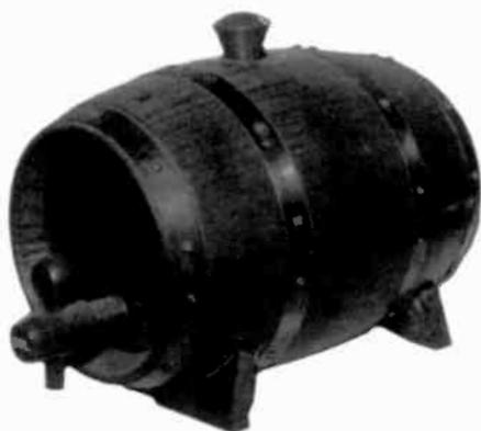
**KEG NOVELTY RADIO** – This 6-transistor radio in the shape of a wine barrel was manufactured in Japan. It operates on a 6-volt battery. The keg tap is the on/off/volume switch, and the top plug is the tuning knob. (*John Phipps – St. Charles, MO*)
