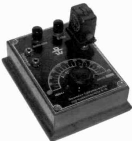
**DTW TYPE D.E. 3** – This German Crystal set has seven different plug-in crystal units. It was manufactured in 1926 by Deutsche Telephonwerke and Kabelindustrie A-G. The front panel is aluminum. (Erwin Macho – Vienna, Austria)
