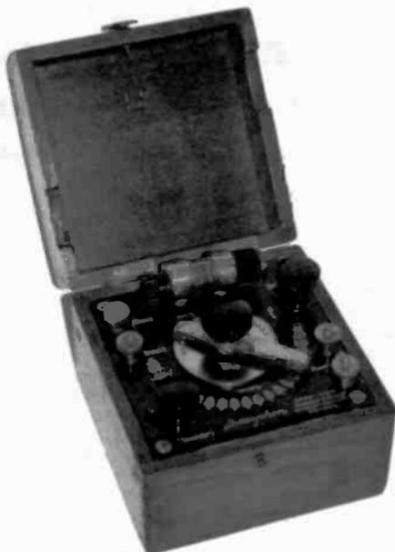
**BRUCKNER "LUMOPHON" TYPE D CRYSTAL SET** – Made in Nürnberg, Germany, this 1924 crystal set is maybe one of the best German-made sets. It has condenser and coil tuning and still has its original crystal detector. A highlight of my collection! *(Erwin Macho – Vienna, Austria)*
