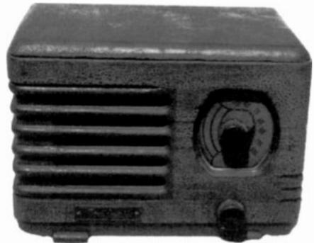
**MARSHALL, MODEL UNKNOWN** – This 4-tube, wooden radio is very similar to the Detrola Model 440. The following tubes are used: Types 6A8, 6J7, 25L6 and 25Z6. The cabinet finish and resistance line cord are original. The filter caps were replaced, and it works fine. It was found at a local garage sale. (*Max Stephenson — Port Clinton, OH*)
