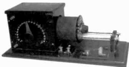
**REPLICA LOOSE COUPLER RECEIVER** – This is a reproduction of a 1912 crystal set built in 1969 by Bob Herbig of Oceanside, California. It uses a Navy-type loose coupler, Murdock phone condenser and a catwhisker-type crystal detector. The board measures 16½" long. (Wally Worth – Wollaston, MA)
