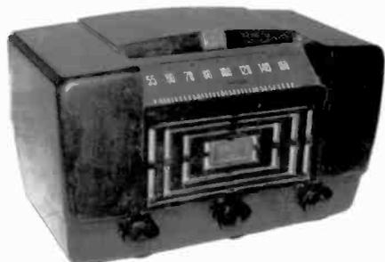
**RCA VICTOR MODEL 66X11** – This brown plastic radio was sold in 1947. It has a 6-tube, AC/DC chassis and plays the broadcast band only. (Clark Trissell – Lincoln, NB)
