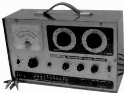
**B&K MODEL 960** – Your transistor radio not working? Use this B&K Model 960 transistor radio analyst to check it out. It provides eight separate DC voltages, an individual transistor checker for in- or out-circuit testing, a VTVM, an output meter, and an RF/IF signal generator. (Ray Chase – Plainfield, NJ)
