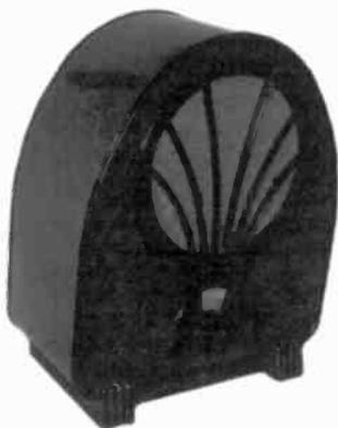
**PHILIPS MODEL 830A** – This 5-tube "Superinductance" is of a hi-tech TRF design, having very complex components. The Litz-wound coils have glass formers in huge copper cans. The laminate "Arborlite" cabinet is over a steel frame. (*Jim Taylor – Bournemouth, England*)
