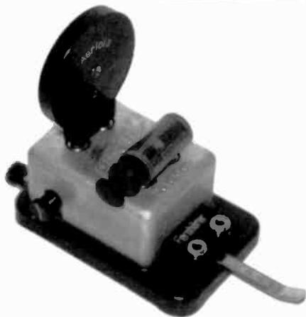
**SCHUCHARDT ALLRATOR CRYSTAL SET** – I looked for about 20 years for this most wanted set and finally bought it in 2002 in Sweden. Made in 1926 in Germany, it has condenser tuning (see the small lever), a plug-in detector from Selectit, and an Aeriola coil. It receives both long and short signals. (Erwin Macho – Vienna, Austria)
