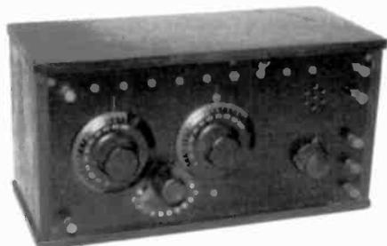
**SHEPCO RECEIVER** – This "all-purpose" receiving set was manufactured by the Shepard-Potter Co. of Plattsburg, N. Y. It sold for \$21 in 1924. The instructions claim that the set may be used in innumerable circuits by interchanging jumpers to terminals at the top and on the inside of the panel. (*Leonard Aquino – Putnam Valley, NY*)
