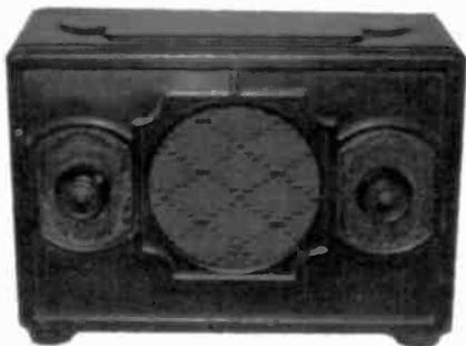
**GENERAL ELECTRIC MODEL BX** – This small, metal-cased radio was manufactured in 1932. The 4-tube chassis contains a voltage-dropping filament resistor. (*Jack LaVelle – Oak Forest, IL*)
