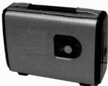
**KOLBERG TYPE R3** – This battery-operated portable has three bands — long wave, broadcast and shortwave. It uses five miniature tubes and can be operated on AC using a separate adapter cord. I believe the set was manufactured in Norway by the Kolberg Skagmo Co. (Ray Chase – Plainfield, NJ)
