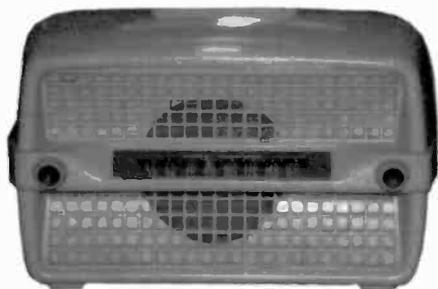
**PHILCO TRANSITONE MODEL 49-505** – This ivory plastic table model set was manufactured in 1949. Operation is AC/DC with 5 tubes, and it tunes the broadcast band. It has a checkerboard design front with a molded handle on the top surface. (*Michael Comer – Haslett, MI*)
