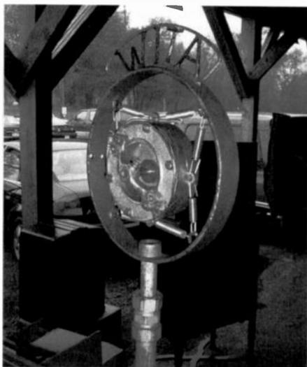
Radio Station WITA spring-type microphone.
