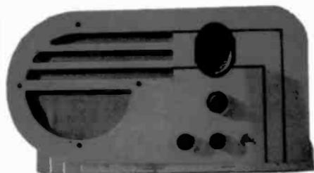
**PHILCO MODEL 610** – This 3-band table radio, manufactured in 1936, has the following five tubes: (1) Type 6A7 detector/oscillator, (1) Type 78 first IF, (1) Type 75 second detector/first AF, (1) Type 42 output, and (1) Type 80 rectifier. A supplement to the Philco Bulletin No. 217 indicates that the Model 610 was a 1935 production run. (*Ray Schneider – San Leandro, CA*)
