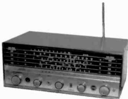
**HALLICRAFTERS MODEL S-120** – This 1950s shortwave receiver has four bands and operates on AC/DC with the following tube types: 12BE6, 12BA6, 12AV6, 50C5, and a selenium rectifier. It has a ferrite loop for broadcast reception and a telescoping antenna for the shortwave bands. (*Clark Trissell – Lincoln, NB*)
