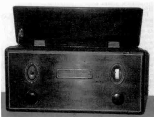
*Figure 1. A front view of the RCA Radiola 16. The symmetrical arrangement of controls includes a volume control, lower left, a tuning control, lower right, and the on/off switch, upper left. The tuning dial is located above the tuning knob.*
