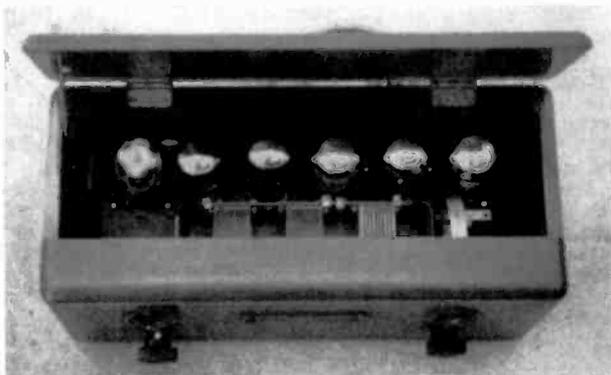
*Figure 2. An inside peek shows the six tubes and the tuning capacitor.*
