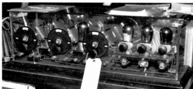
Above: A radio with a view. This 5-tube home-brew Neutrodyne is housed in a glass case. Left: Two Von Lieben LRS relay tubes. The tube on the left, with an open filament, sold for \$7,000. The clear glass tube, with a good filament, right, sold for \$14,500.
