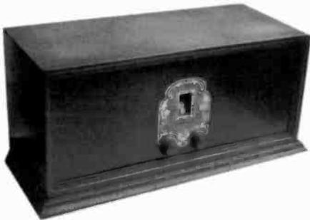
**MURDOCK MODEL 65** – This "single dial tuning" receiver was manufactured by the Wm. J. Murdock Co. of Chelsea, Mass. It uses six Type 201-A tubes and a Type 71 output tube. In 1927, it sold for \$65. (Ray Chase – Plainfield, NJ)
