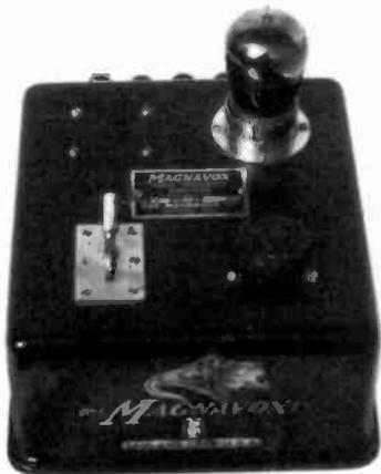
**MAGNAVOX TYPE A1** – This 1-tube amplifier in a metal case sold for \$27.50 in 1923. The tube being used here is a rainbow Type 201-A. (Ross Mason – Mason City, IA)
