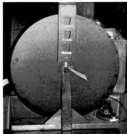
*A different kind of home brew — a mechanical TV scanning disc and motor mounted on a wooden frame.*
