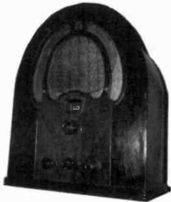
**PHILCO MODEL 60B** – Because Philco was one of the leading radio manufacturers of the 1930s, the company made many different cathedral styles. However, this is one of the classic 1934 designs offered with the revolutionary 5-tube superheterodyne chassis. (Carl D. Sutton – Ironton, OH)
