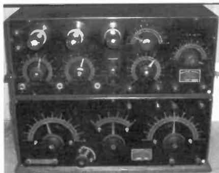
Below, a Chicago Radio Labs PAR tuner; above, a Model AGN-2 detector/2-stage amplifier.
