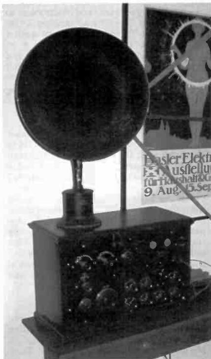
A Federal Model 61 driving a large Federal horn was playing during the open house using an ARBE-III battery eliminator.
