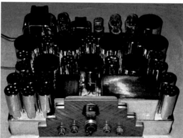
Figure 1. A front view of the 23-tube Scott Full Range High Fidelity receiver.
