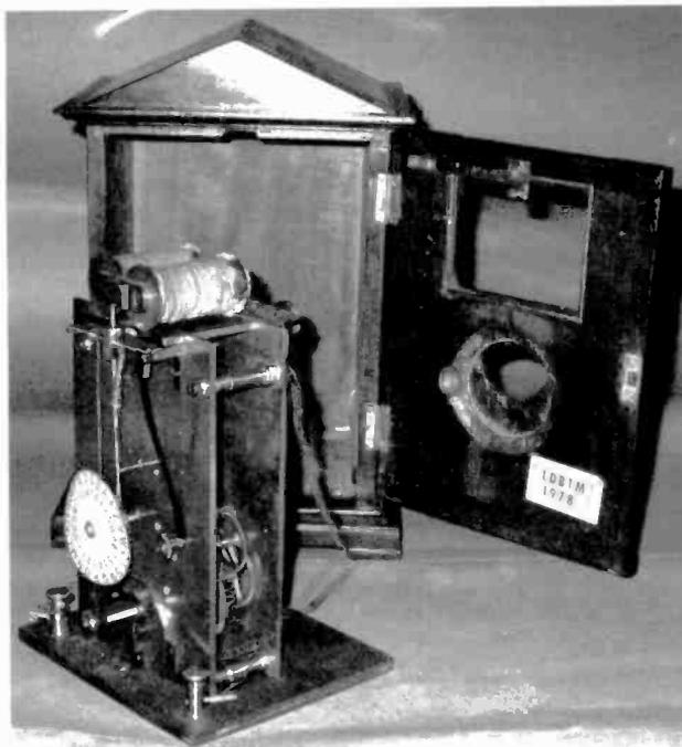
An internal view of the Cooke and Wheatstone ABC Telegraph Receiver. The mechanism consists of a spring driven clockwork, controlled by an electromagnetic escapement. This escapement is actuated by the pulses of current from the sender and allows the dial to rotate one letter for each letter passing the index on the sender apparatus. The dial on the receiver moved in unison with the dial on the transmitter and the disc of paper displayed the correct letter.
