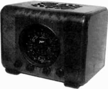
**ZENITH MODEL 6S222** – This set, manufactured in 1937, is one of the many "big black dial" radios of that era. It has a 6-tube chassis, and because of its cube shape, the speaker grille is on the top. It tunes both the broadcast and shortwave bands. (*Clark Trissell – Lincoln, NE*)
