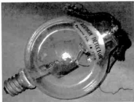
De Forest Wireless Company Single Wing Audion vacuum tube, 1909. This was the first commercial, 3-element vacuum tube placed on the market, and it enabled wireless signals to be amplified for the first time. This tube is complete with good filaments and original label.
