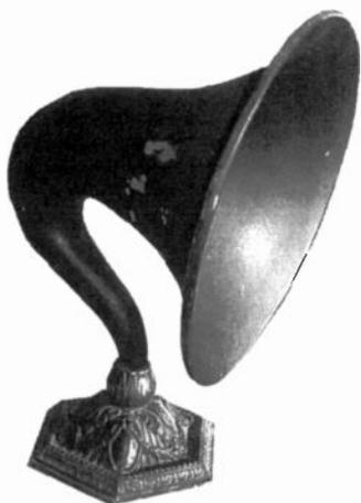
**STEWART-WARNER MODEL 400** – This horn speaker was manufactured by the Stewart-Warner Speedometer Co. of Chicago. The 15" diameter fiber bell sits on a heavy cast metal "tulip-styled" base. Its original price was \$25. (Dave Crocker – Mashpee, MA)
