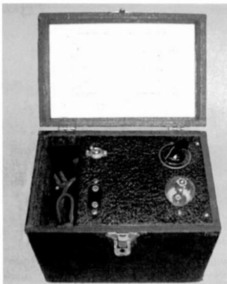
Figure 1. T&H Manufacturing's Model 60 Analyzer is an example of an early capacitor test set.
