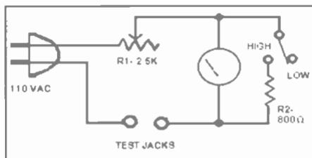
Figure 5. This schematic diagram for the Readrite Model 800 reveals the tester's simplicity.
