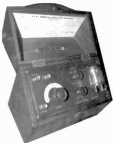
**B.T.H. WIRELESS RECEIVER** – This 1923 crystal set was manufactured by the British Thomson Huston Co., Ltd., of London. It has a unique twin crystal detector, both of which are enclosed in a single celluloid mount. (Jim Taylor – Bourmemouth, England)
