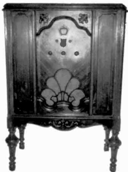
**MIDWEST, MODEL UNKNOWN** – This 9-tube, multiband console was manufactured around 1932 by the Midwest Radio Co. of Cincinnati, Ohio. The paper labels are missing, but Serial #C-13725 is stamped on the chassis. (Carl D. Sutton – Ironton, OH)
