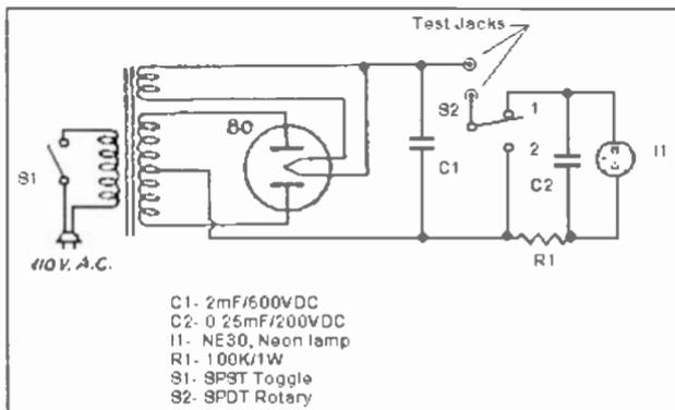
Figure 2. A schematic diagram of the Model 60 tester. Note the presence of high voltage at the test terminals.
