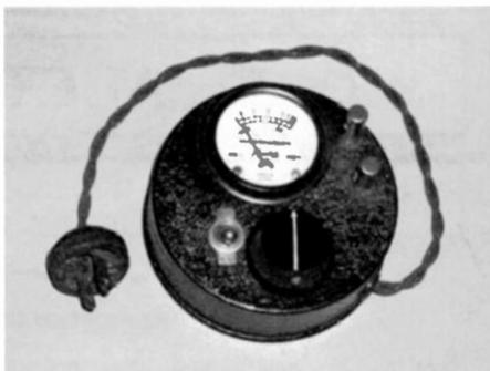
Figure 4. A Readrite Model 800 direct-reading capacitance measuring device. Line voltage appears at its test terminals, and the unit lacks an on-off switch.
