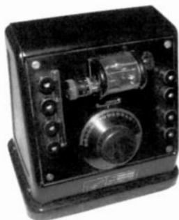
**ISARIA TYPE D CRYSTAL SET**– This rare crystal set was manufactured by Isaria Zählerwerke in 1924/25. It is a German set with variometer tuning and a black metal case. The plug-in crystal detector is called "Red Star," a very expensive component. (Erwin Macho – Vienna, Austria)
