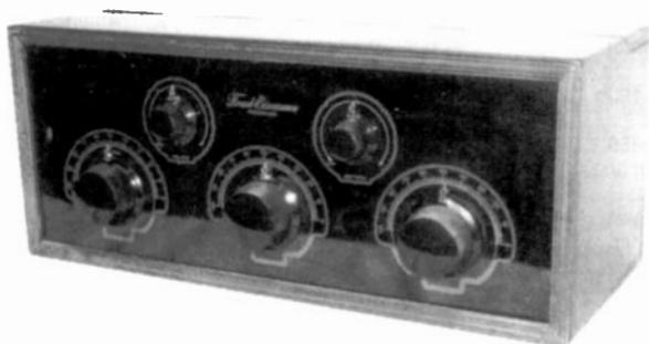
**FREED-EISEMANN MODEL 10** – This 5-tube battery receiver was manufactured in 1926 in New York City by the Freed-Eisemann Radio Corporation. It uses Type 201A tubes in its Neutrodyne circuit. (Wally Worth – Wollaston, MA)
