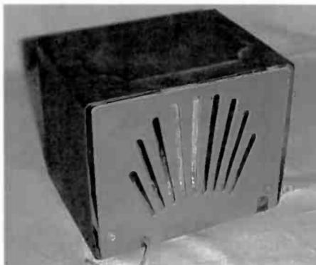
Figure 3. This rear view of the radio shows the replicated rear cover.
