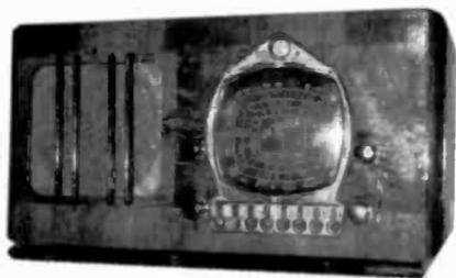
**DETROLA MODEL 175E** – This rather large 1937 table set has the tuning capabilities of the "Big Dial" consoles. It measures 21" wide. A 10-tube radio with motorized push-button tuning, it receives two shortwave bands and the broadcast band. (Carl D. Sutton – Ironton, OH)
