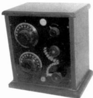
**1-TUBE RECEIVER, MANUFACTURER UNKNOWN** – This very small, 1-tube radio is a mystery. Inside is a variable plate tuning condenser and a tapped variocoupler with spiderweb coils. A rheostat, tube socket, phone jack, and Fahnstock clips complete the circuit. Can anyone identify this set? (Wally Worth – Wollaston, MA)
