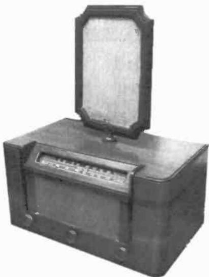
**TRUETONE MODEL D-2121** – This 5-tube, wood cabinet set was manufactured in 1958 for Western Auto Supply of Kansas City, Missouri. It is a battery-operated radio for farm use and has a rotatable external antenna on top of the cabinet. (C.R. "Ron" Lawrence – Matthews, NC)
