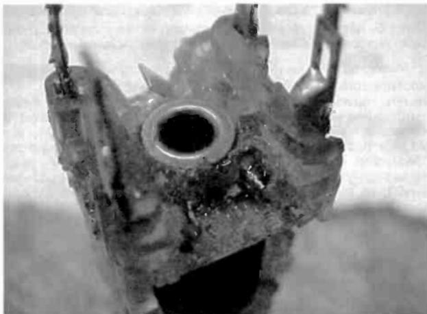
Figure 3. This view shows one of the tabs lifted (rear) and one section of the mica capacitor removed (foreground).
