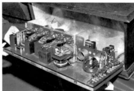
An interior view of the mystery radio. The modified 4D chassis is on the left, and an amplifier with one of the Western Electric tubes is on the right.
