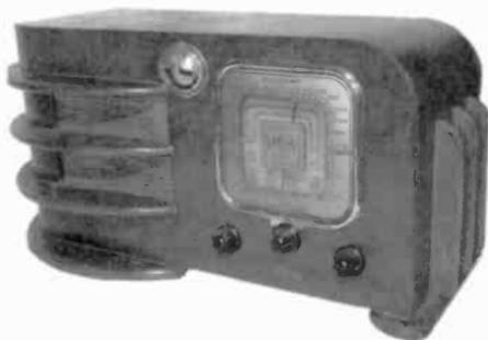
**GENERAL TELEVISION, EMERALD MODEL** – This all-wood cabinet radio, ca. 1939-1940, was built by the General Radio and Television Corp. of Chicago. It has a 6-tube circuit with a bias cell. The tuning eye tube is a Type 6G5. It tunes both the broadcast and shortwave bands. A smaller version was named the "Baby Emerald." (Jim Knapp – Phoenix, MD)
