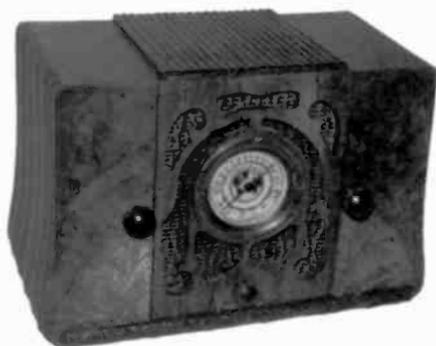
**DETROLA MODEL 240** – This stylish 1938 table radio was manufactured by the International Detrola Corp. of Detroit, Michigan. The 5-tube chassis uses the following tube types: (1) 6A7, (1) 6D6, (1) 75, (1) 47, and (1) 80 rectifier. This restored model may not have the original knobs. (*Clark Trissell – Lincoln, NE*)
