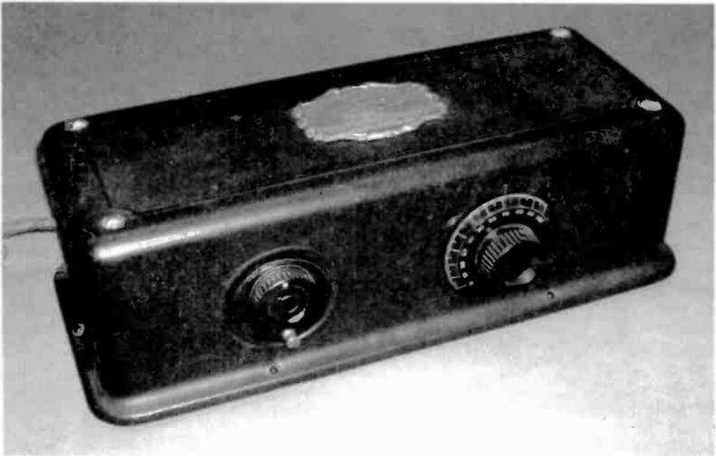
*The Atwater Kent Model 35, a 6-tube TRF, was introduced in 1926, and is commonly referred to as the "bathtub set."*
