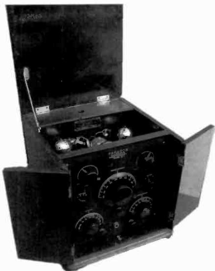
**PARAGON TYPE III-A** – This rather compact receiver was manufactured in 1924 by the Adams-Morgan Company of Upper Montclair, New Jersey. It is a 3-tube receiver about which Alan Douglas' *Radio Manufacturers of the 1920's* says is a repackaged version of the Paragon Type RB-2 of 1923. It has two doors and a top cover lid, all of which when closed make it look like not much. Nevertheless, it is a rare set. (Dave Crocker – Mashpee, MA)
