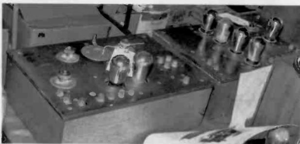
*This unusual Westinghouse 2-tube receiver and its companion 5-tube amplifier sold for \$4,200. In 1924, Westinghouse utilized units like these to receive KDKA's programs at other Westinghouse network stations for rebroadcast. These units were also used to receive the program for the Westinghouse Founder's Day Banquet on October 12, 1924, at which 7,000 people dined in 62 different cities.*
