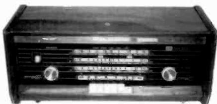
**PHILIPS MODEL B5X43A** – Found sitting curbside on the grass in the rain with a take-me-home look, this attractive, early 1960s LW/BC/SW/FM stereo receiver is a hybrid design with 10 tubes plus a 6-transistor stereo decoder. It is switchable between six different line voltages from 110 to 245 VAC, uses 800-ohm speakers, and has wonderful sound quality. (Chris Jones – Fairport, NY)
