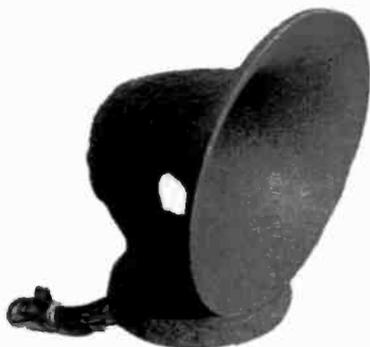
**TEMPLE REPRODUCER** – This one-piece horn speaker is made of molded fiber, even though the manufacturer called it a "ceramic" material. The driver is mounted in the bottom. The color is a "speckled" or "mottled" green. It is extremely lightweight. The manufacturer was the Chicago Signal Company for Parcells & Company, also of Chicago. In 1925, it sold for \$21. (Dave Crocker – Mashpee, MA)
