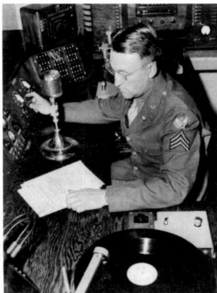
Figure 4. This photograph of Scribner at the PBS control panel provides some details of the equipment. The control panel is custom-built, the Shure microphone and the RCA transcription turntable are typical commercial items of the period. Other commercial items include an intercom, upper left, and an RCA BC/SW receiver, top.
