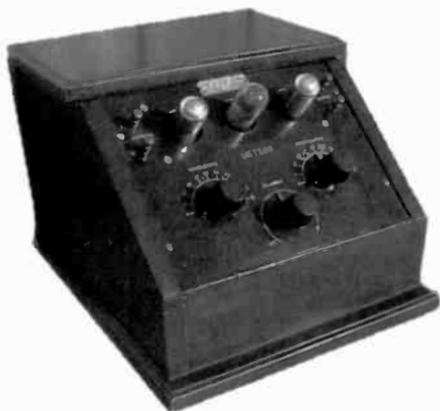
**METEOR MODEL V3** – Measuring only 9" tall, this 1924 receiver uses three Type UX-199 tubes. It was manufactured by the Radio Shop of Long Beach, California, and sold for \$50. The top cover lifts for inserting batteries for the 199 tubes. (Dave Crocker – Mashpee, MA)
