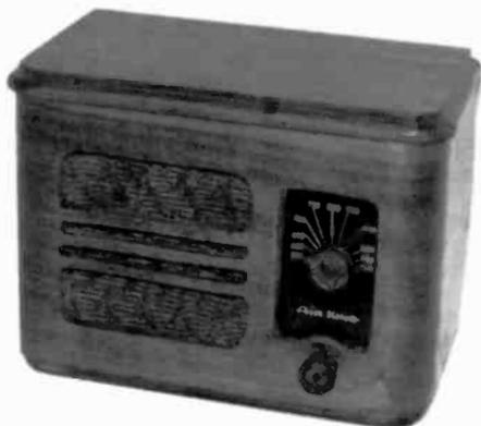
**AIR KING MODEL 1001** – Manufactured by Air King Products Co., Inc., Brooklyn, New York, this tiny wooden-cabinet radio has a 4-tube chassis using the following tube types: (1) 6D6, (1) 6C6, (1) 43, and (1) 25Z5. (Clark Trissell – Lincoln, NE)
