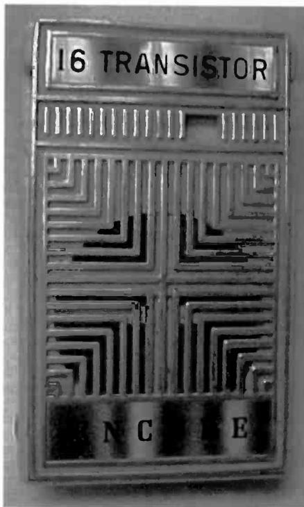
Figure 1. The Encore 16-transistor pocket radio.
