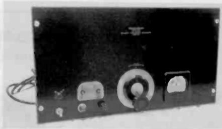
Figure 1. A front view of the Western Electric Primary Frequency Standard shows the controls and connectors, including the precision tuning dial and meter.
