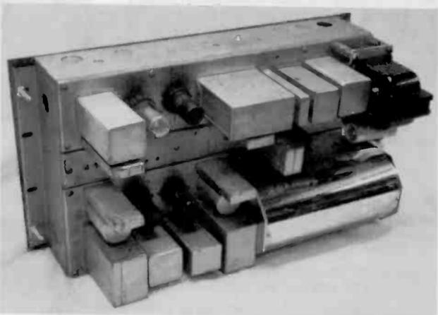
Figure 2. A rear view of the Frequency Standard shows the neatly arranged components and tubes. The crystal oven is the shiny chrome-plated device in the lower right.
