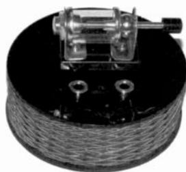
**MOTALAREN** – This crystal set was made in Sweden. It is an outstanding design built in a coil and using a plug in-detector, which was also made by a Swedish company called EKA. (*Erwin Macho - Vienna, Austria*)
