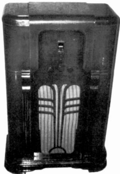
**PATTERSON, MODEL UNKNOWN** – This 17-tube, 4-band console, was manufactured by the Patterson Electric Co., ca. 1934. Patterson was more widely known for military and Amateur receivers. The set was advertised in our local newspaper as a "1920s, floor model transistor radio in very good condition." I was glad to relieve the owner of what he called, "this old thing." (*Carl D. Sutton – Ironton, OH*)
