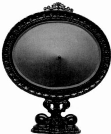
**SPLITDORF CONETONE** – This elliptical paper cone was manufactured in 1927 by the Splitdorf Radio Corporation of Newark, New Jersey. It was offered as a companion speaker to the Splitdorf Abbey radio. It has a wooden back and sits atop a papier-mâché stand that swivels. It stands 26" tall and 22" wide. (Ross Mason – Mason City, IA)
