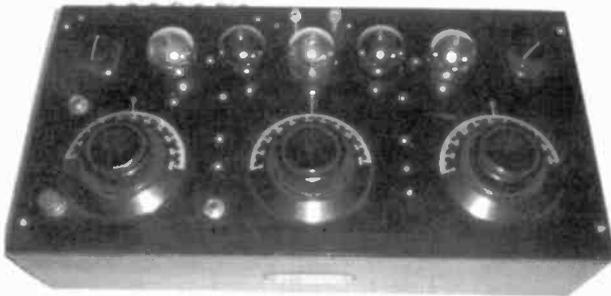
**PANDORA, MODEL UNKNOWN** – This 5-tube TRF battery radio was made by John Lurie, Jr., of New York, even though it was found in Australia. The serial number is left blank on its oval nameplate. The cabinet is leatherette-covered wood and stands only 5 1/2" high. The battery terminals are mounted on the rear of the cabinet. Is anyone familiar with this receiver or its manufacturer? (Richard Begbie – Bungendore, Australia)
