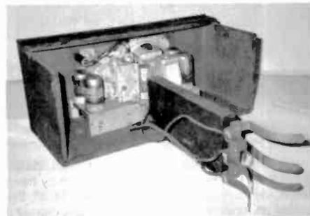
Figure 4. The three pairs of contact "fingers" are shown on the lower right in the photo above.
