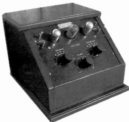
**METEOR MODEL V3** – This 1924 receiver uses three Type UX-199 tubes. It was manufactured by the Radio Shop of Long Beach, California, and sold for \$50. It measures only 9” tall. The top cover lifts for inserting batteries for the 199 tubes. *(Dave Crocker – Mashpee, MA)*
