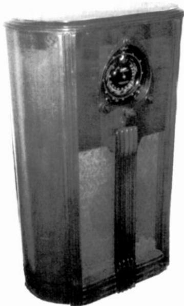
**ZENITH MODEL 9S263** – Housed in an unusual oval-shaped cabinet, this 1938 console uses a 9-tube shutter dial chassis with a tuning eye. The tuning range is 500 kHz to 18 MHz. *(Tom Ackerman – Germantown, IL)*
