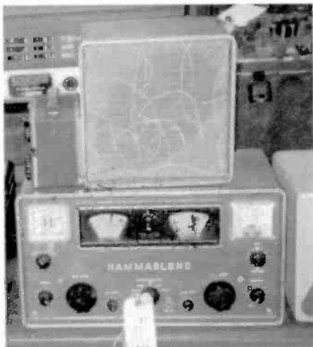
This Hammarlund Model HQ-110 is a 12-tube receiver that tunes seven Ham bands from 160 to 6 meters. In good condition, it sold for \$120. This set has a matching speaker but no clock.
