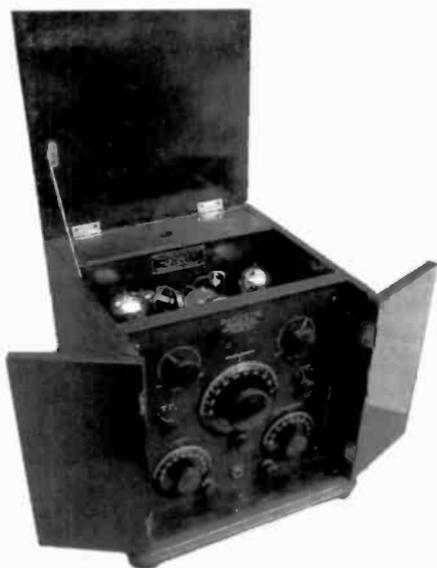
**PARAGON TYPE III-A** – This rather compact receiver was manufactured in 1924 by the Adams-Morgan Company of Upper Montclair, New Jersey. It is a 3-tube receiver, which Alan Douglas' *Radio Manufacturers of the 1920s* says is a repackaged version of the Paragon Type RB2 of 1923. It has two front doors and a top cover lid, all of which, when closed up, don't look like much, but it's a rare set, nonetheless. (Dave Crocker – Mashpee, MA)
