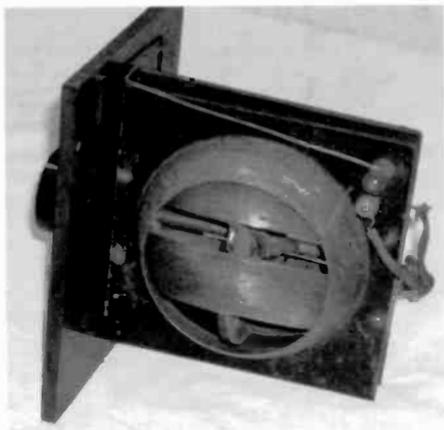
Figure 3. An interior view of the Type SR-23 variometer.
