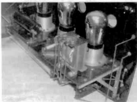
Figure 12. This close-up of the SR-21 chassis shows some of its components, including the interstage audio transformer and a Federal coil.
