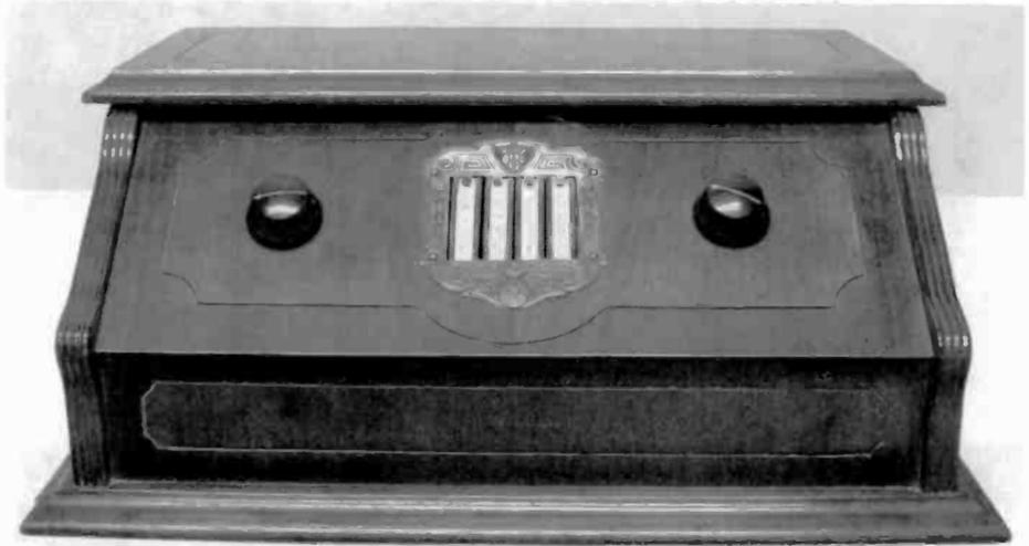
Figure 15. A front view of the 7-tube Model 77 radio. Tuning is accomplished by the four thumbwheel knobs.
