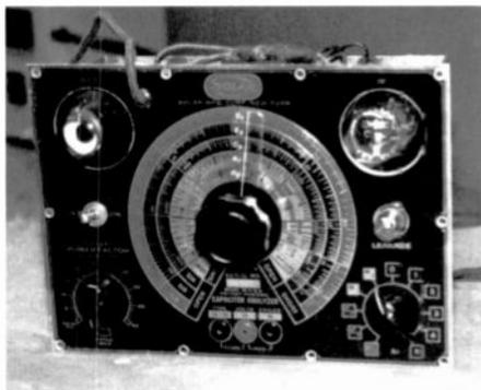
Figure 3. This Solar Model CB, an early Resistance-Capacitance Bridge, uses a Type 6E5 eye tube as an indicator and a Type 1V as a rectifier.
