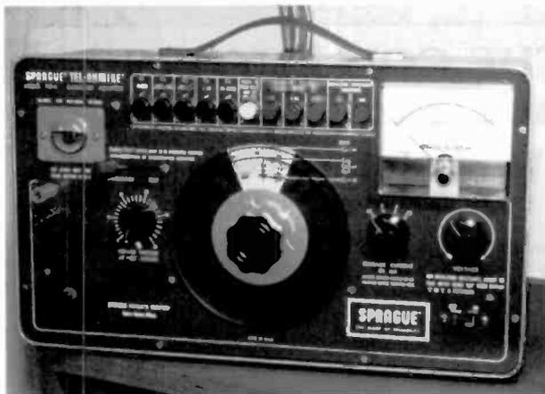
Figure 14. This Sprague Model TO-6 "Sprague Tel-Ohmike" capacitor analyzer uses push buttons to select capacitance scales and test voltages. The analyzer is easy to use. I use it to reform electrolytic capacitors.
