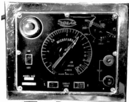
Figure 4. A front view of the Model QCA. It was the first Solar tester with the "Quick-Check" feature.
