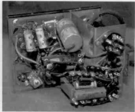
Figure 7. A rear view of the chassis for the BQC shows tight but neat packaging.
