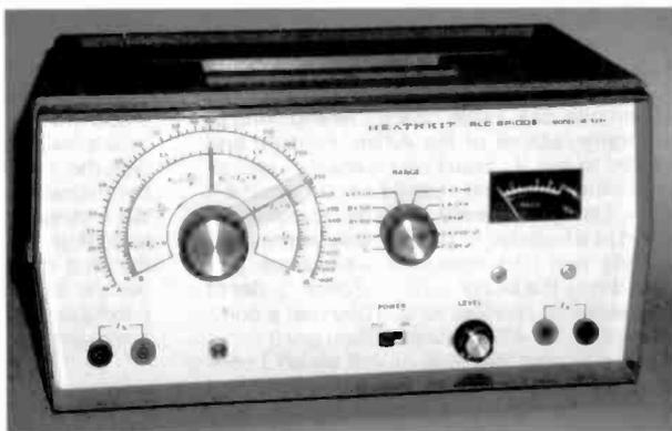
Figure 15. Just one of the many Heathkit capacitor testers and capacitor substitution boxes sold in kit form, this RLC Bridge, Model IB-5281 is a battery-operated, solid-state instrument.
