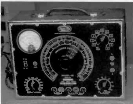
Figure 8. The first Solar Exam-eter, the Model CE "Capacitor Analyzer," used the term "Exam-eter" in the user's manual, but it did not appear on the panel. It was the first Solar analyzer to use a meter rather than an eye tube.
