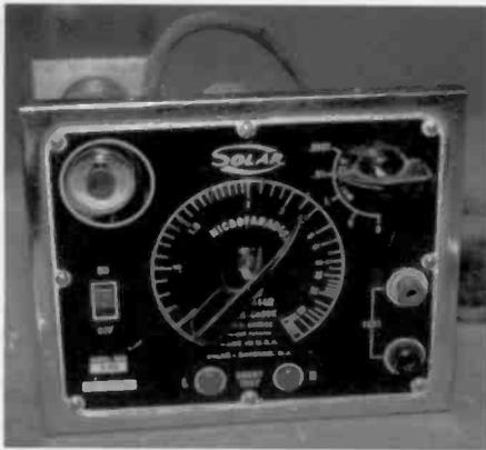
Figure 6. The Solar Model BQC is similar to the QCA but is housed in a smaller cabinet. Also, push buttons are used for the Short Test while the QCA uses slide switches.
