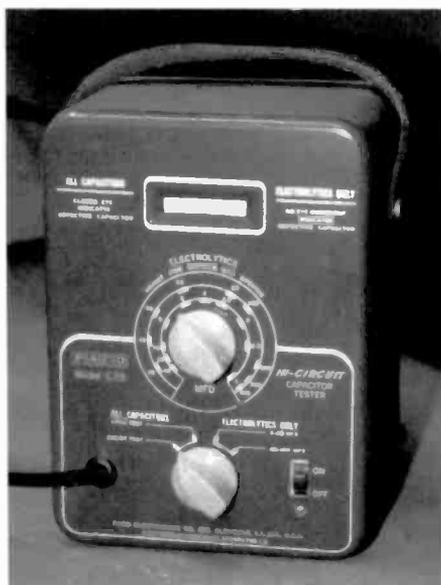
Figure 12. This PACO Model C-25 "In-Circuit Capacitor Tester," uses a modern Type EM84 tube as an indicator. It sold for \$19.95 as a kit or factory wired for \$29.95.
