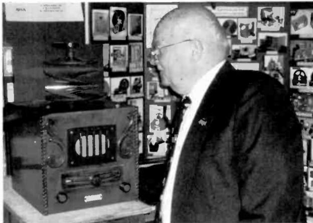
Peter Yantzer, right, demonstrates his early mechanical television apparatus that uses a rotating, spiral, segmented mirror. A picture produced by the TV is shown on the left.
