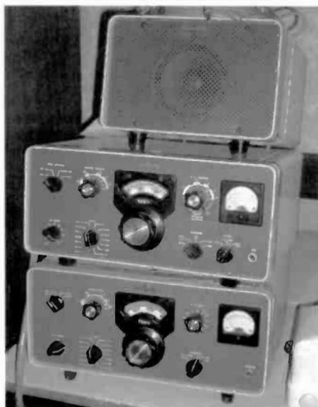
Ready to plug and play, and selling for only \$800 — a Collins "S-Line" station consisting of a 75S-1 receiver, a 32S-1 transmitter, as well as a power supply/speaker, cables and a user's manual.
