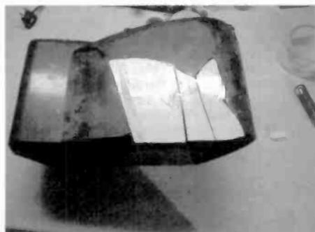
Figure 2. A replacement piece of Bakelite has been cut to size and taped in place on the top.
