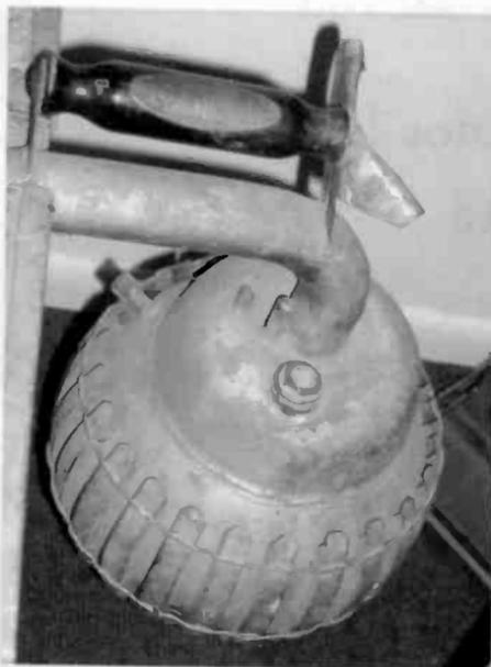
Figure 3. A close-up of the Icyball's pressurized vessel, or "hot ball," that was heated by a flame.
