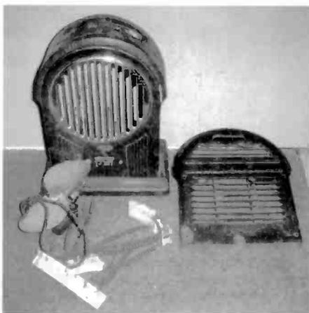
Figure 3. The Sunbeam heater after disassembly. Shown are the metal cabinet, rear panel, fan, and heating elements.
