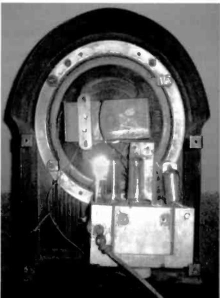
Figure 11. This rear view shows the finished project with the chassis and speaker mounted in the cabinet.
