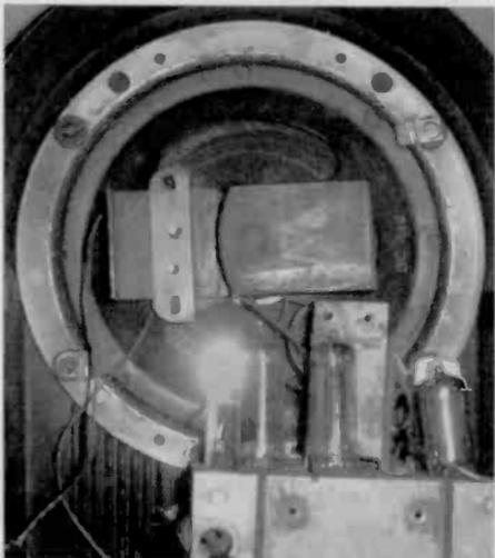
Figure 6. The PM speaker is attached to the cabinet's chrome housing in two places.
