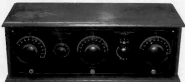
Figure 8. The 1926 version of the Model TR-5 uses four Type 01-A tubes and one Type UX-112.
