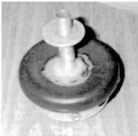
Figure 6. The driver unit with its mounting hardware in place.
