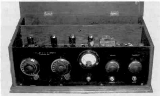
Figure 4. This Hallock and Watson 8-tube superhet used Type UV-199 tubes and a meter to monitor filament voltage.
