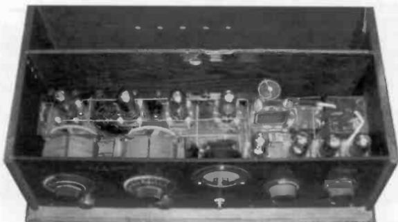
Figure 5. This top view of the 8-tube superhet shows the component layout and bus bar wiring.
