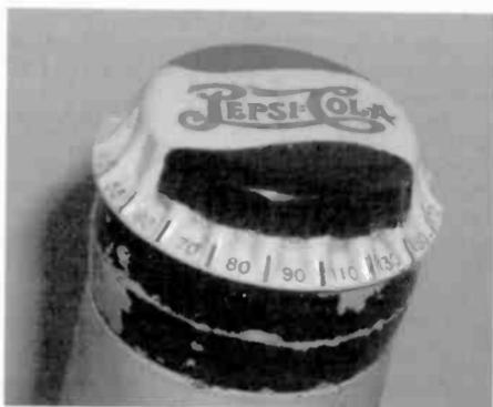
Figure 2. Here is a real "tuning cap." The calibrated bottle cap serves as the tuning dial.
