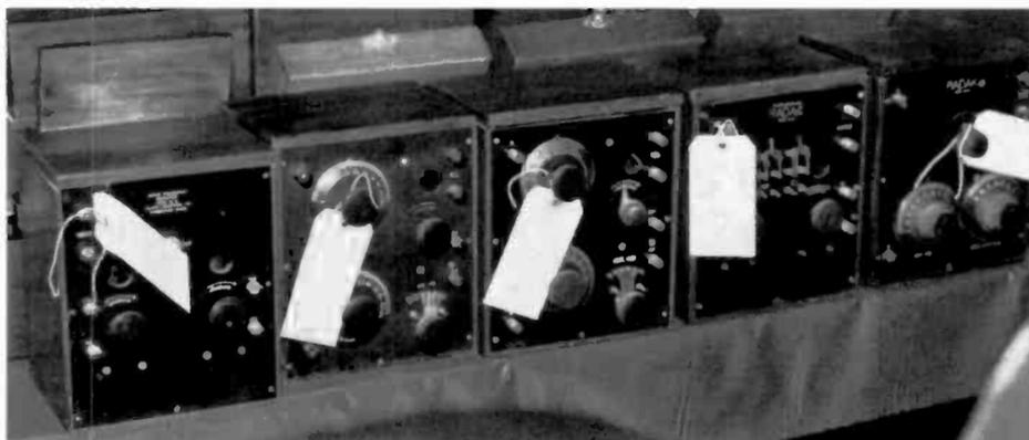
A line-up of Clapp Eastham sets: Left to right, HZ, 2-step audio amplifier (phono-jack version); RZ, 1-tube receiver; HR, 1-tube receiver; HZ, 2-step audio amplifier (knife switch version); and R4 receiver.
