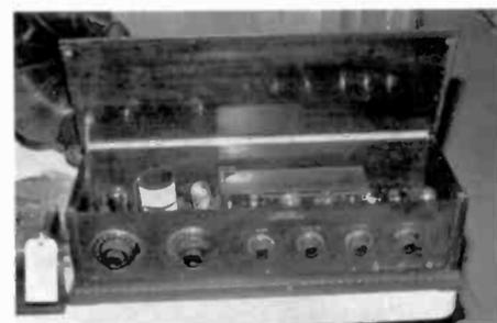
An 8-tube Master superhet complete with tubes. The IF transformers are housed in the wooden enclosure at the rear of the set's cabinet. This set may have been manufactured by the Chicago Radio Labs. It sold for \$400.
