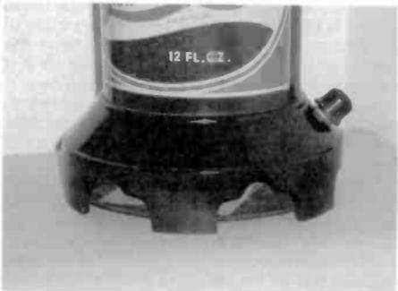
Figure 3. The radio's base shows the cardboard disk that protects the speaker and serves as a sound diffuser. Note the volume control on the right side.
