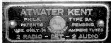
Comparison of a standard Atwater Kent Model 20 tag, above, with that of the Model 5A, below. Note the Model 5A tag specifies the tube functions: "2 RADIO - DET. - 2 AUDIO."
