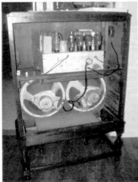
*Figure 3. A rear view of the Model 344 showing the twin speakers and the chassis.*
