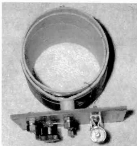
Figure 5. A side view of the tuning coil showing one winding inside the larger winding.
