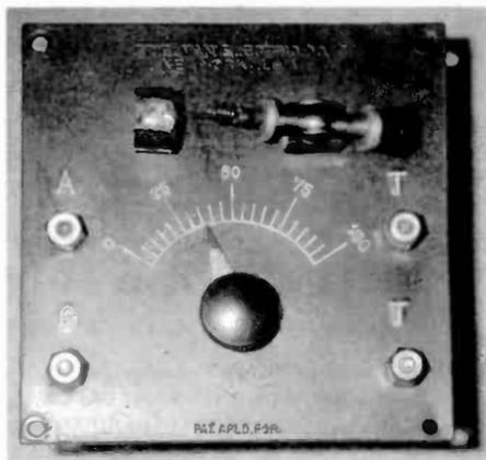
Figure 3. A close view of the crystal set panel showing the crystal, the tuning knob and the binding posts for antenna, ground, and telephone (or phones).
