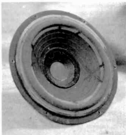
Figure 3. The highly compliant suspension of the speaker is visible in this photograph.
