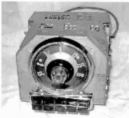
Figure 1. A front view of the radio from a 1950 Ford showing the concentric tuning and volume controls, and the five push buttons.
