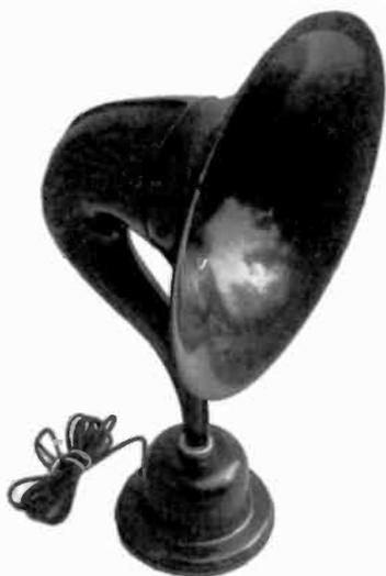
**MAJESTIC GGH MODEL WG-10** – Manufactured by the Grigsby-Grunow-Hinds Co, this horn speaker has a metal base with black Pyralin (celluloid) upper horn and neck. The horn's diameter is 12½" and the speaker stands 22" tall. Other celluloid models were offered in mahogany, Japanese pearl and mother-of-pearl. (John Drake – Madison, CT)
