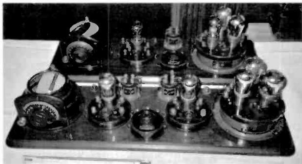
*Merrill Bancroft's entry in the TRF contest category was two of the earliest factory assembled Atwater Kent breadboards. The Model 4052, rear, has one stage of RF amplification, a detector, and two stages of audio amplification. The Model 4066, front, the first Atwater Kent set with five tubes, has an additional stage of RF amplification.*
