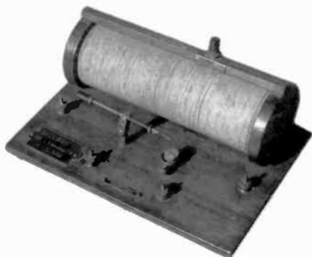
**CASA MONTES CRYSTAL SET** – This rather unusual crystal radio was manufactured in Spain by Casa Montes of Madrid. It has the unique double-swivel detector with catwhisker-type wire. The slide tuner has cotton-covered wire. The hardware, including the nameplate, is all brass. It measures 8¼" x 5½" at the base and stands 4¼" tall (David Pope – Plymouth, MA)
