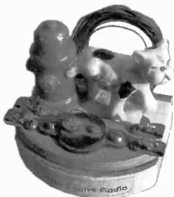
**LITTLE SQUIRT CRYSTAL SET** – This unique crystal set was fabricated by a radio collector with imagination. The detector is an inexpensive catwhisker type missing the glass dome. The Fahnestock clips and an adjustable, "squeezeable" coil of wire were all mounted to a ceramic base depicting a little Bulldog using the services of a bright red fire hydrant. The complete unit measures less than 3" wide x 2½" tall. (David Pope – Plymouth, MA)
