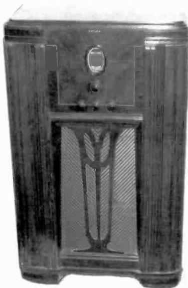
**PHILCO MODEL 630X** – This 6-tube console was manufactured in 1936 by the Philco Storage Battery Company of Philadelphia, Pennsylvania. It tunes broadcast and shortwave bands. (Clark Trissell – Lincoln, NE)
