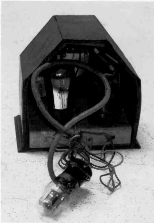
Figure 5. Connections between the adapter and the radio are made using the cable and wafer tube socket shown in this photo. The external tube is the detector tube from the radio.
