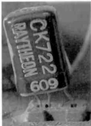
Figure 4. A Raytheon CK722 transistor and socket.
