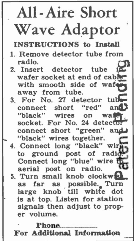
Figures 8. The label on the All-Aire short-wave adapter.
