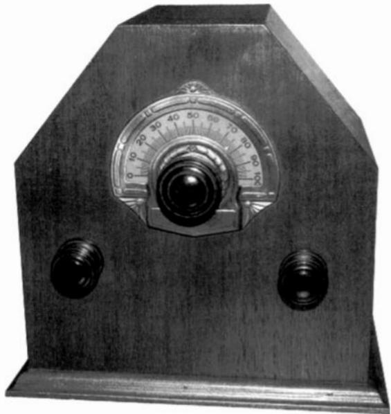
*Figure 1. The Shorty model shortwave adapter is distinguished by its round knobs.*
