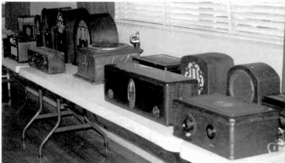
Battery sets, cathedrals, cone speakers, and an acoustic phonograph. In the foreground, right, is an Atwater Kent "coffin" set; to its left is an RCA Radiola 18.
