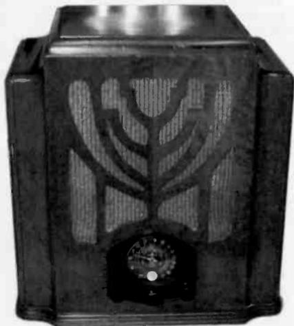
*Figure 1. A Remler Model 88, a hi-fi, 10-tube radio from 1935. It featured a 2-way speaker system and a 15-watt, push-pull output stage using Type 2A3 tubes.*
