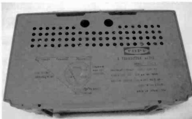
Figure 2. The rear fiberboard cover is full of information, including a dial-stringing diagram — an unusual, but welcome addition.
