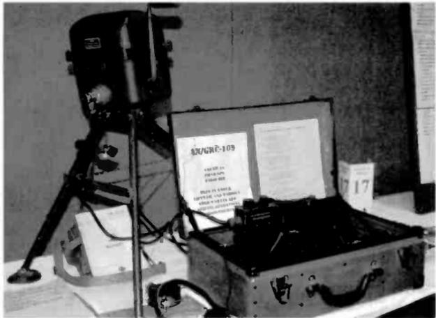
*In the old equipment contest was this AN/GRC-109 American Field/Spy radio set, including a hand powered generator, used for Special Operation assignments and by the CIA.*
