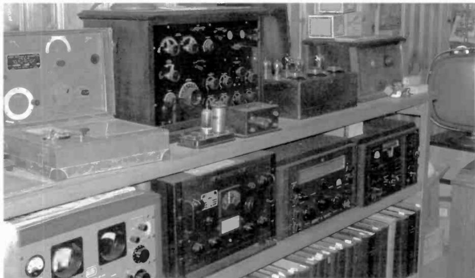
Figure 11. Left to right, top, a BC148, a Federal Model 61, a Dynergy AC set, and a Phanstiehl receiver; Left to right, bottom, a Hammarlund SP-600, a Scott RCH, a Millen DFP 201 and a Millen DFP 501; far right, a Philco Predicta TV — quite a variety of items.
