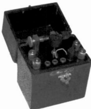
**"LILIPUT" CRYSTAL SET** – "Liliput" was offered in the radio catalog of Vienna Radio dealer Max Böhnel in 1927. It is a very small, impressive Austrian crystal set with variometer tuning and built-in crystal detector. (Erwin Macho – Vienna, Austria)
