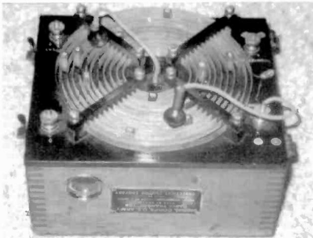
Figure 2. An SCR-65 spark radio transmitter with the original cables.
