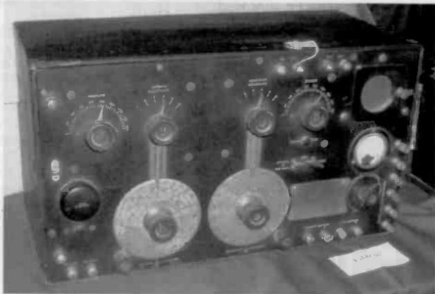
Steve Wallace offered this Medium Wave Receiver, in excellent condition, for \$5,500. The label says that the set was made for the Navy by the American Radio and Research Corp. in 1920 and that its tuning range was 250-7500 M.
