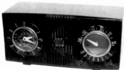
**MOTOROLA MODEL 5C1** – This mahogany, plastic clock radio was manufactured in 1950 by the Galvin Mfg. Co. of Chicago. It is called the "Radio-Larm" and operates on five tubes. (Clark Trissell – Lincoln, NE)
