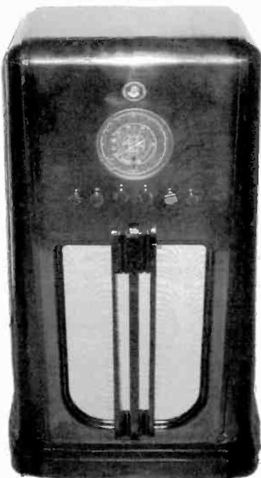
*Figure 1. The refinished cabinet and new grille cloth give this 1937 Fada 290C a fresh-from-the-factory look.*
