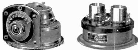
Above, a schematic showing the use of an Atwater Kent coupled-circuit tuner and an Atwater Kent detector-amplifier "TA" unit. Below, the coupled-circuit tuner on the left and the detector-amplifier "TA" unit on the right.
