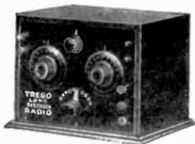
The Trego is a one-tube regenerative set, and is "fully guaranteed for a receiving range of 1,000 miles."
