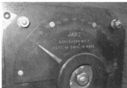
Figure 3. A close-up of the engraving on the panel of the JARS variable condenser: JARS, Condenser No. 7, A, Patt. No. 2486, No. 4956.
