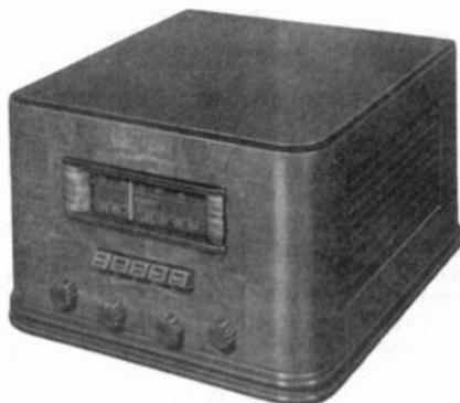
*Figure 1. Crosley recommended the use of its Model 1758A high fidelity, 2-band radio to feed its facsimile printer. The radio tuned the BC band and 24 to 47 MHz band. It featured an amplified AVC circuit to control the radio's output level to the printer.*
