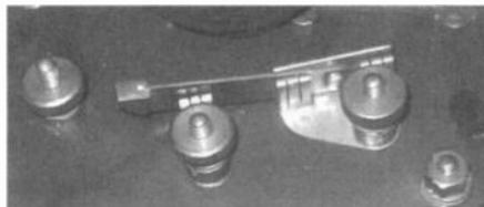
Figure 4. A close-up of the shorting switch on the panel of the JARS variable condenser.
