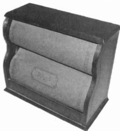
**DICTOGRAND ROLL SPEAKER** – This unusual paper cone speaker was manufactured by Dictograph Products Corp., 220 West 42nd St., New York City. It measures 13½" x 6¾" x 11¼". The Dictogrand reproducer is connected at the center fold of the two paper rolls and has an adjustment screw out the back. The rather thick, parchment-type paper has a gray-brown, mottled finish, and the lettering and edges are embossed. The unit sold for \$16.50 in 1925. (Wally Worth – Wollaston, MA)
