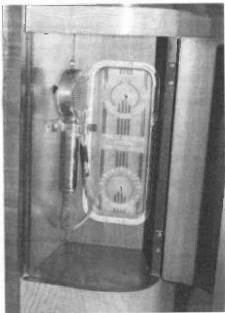
A detailed view of the radio's built-in PA system controls and microphone, an unusual feature even in a high-end set.
