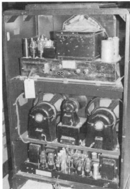
One look at a rear view of the 25-tube Stratosphere and the word "massive" springs to mind. Note the three speakers and heavy-duty amplifier/power supply.
