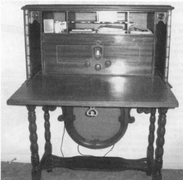
*Figure 6. Richard Arnold's Pooley radio cabinet with the drop-front down showing the American Bosch Model 28 installed.*
