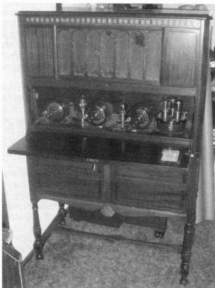
Figure 1. An Atwater Kent Model 10 breadboard in a Pooley cabinet similar to the Model 112-R-2 shown in Figure 3. Unfortunately, there are tears in the grille cloth.
