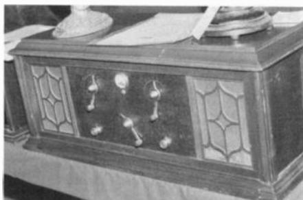
*This Hartman B3 battery set that uses five Type 99 tubes (not included) has a meter for monitoring filament voltage. It sold for \$85.*
