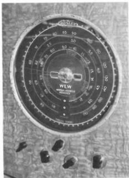
This closeup shows the impressive, large, multi-colored dial used on the Crosley. When tuned to WLW, the WLW call sign in the dial is illuminated.
