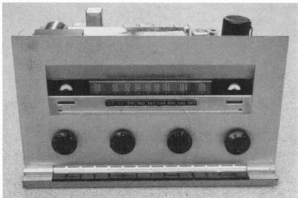
*Figure 2. This front view of the receiver shows its clean lines and symmetrical layout. The front panel was designed by John Vassos. The meters indicate signal strength and FM station centering. Audio bandwidth is graphically indicated on the white line below the bass and treble thumbwheels below the meters.*
