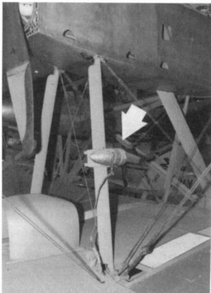
Figure 5. The propeller-driven generator (see arrow) for the transmitter is mounted to the center engine strut.
