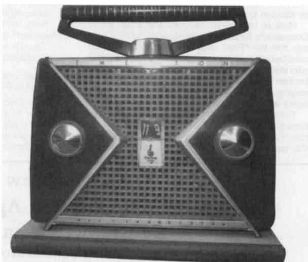
Figure 1. The Emerson Model 847 "All Transistors" with its "Miracle Wand" antenna.
