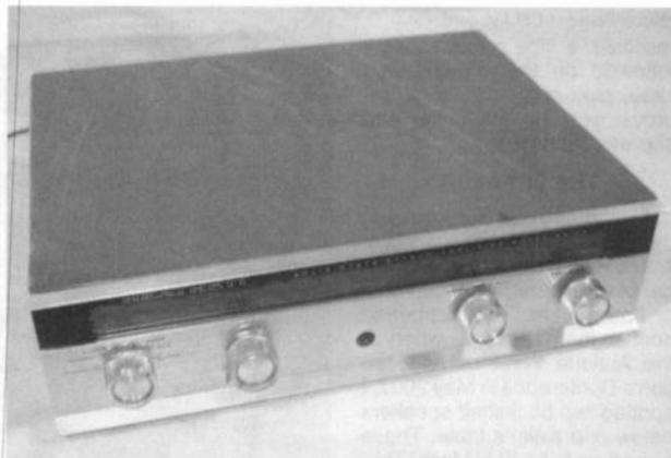
Figure 2. The Heathkit AA-14 provided only source, volume, bass, and treble controls. Speaker and power on-off are push-pull activated by bass/treble controls. The panel is side-lit when on.
