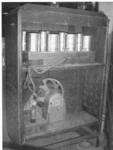
A rear view of the Scott Allwave 15, the two chassis, and the hefty speaker.
