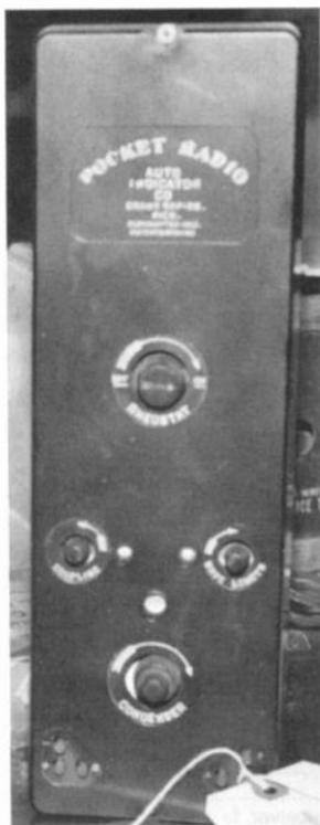
The Pocket Radio, manufactured by the Auto Indicator Co., measures 4" x 12" x 2" deep. The four controls are labeled "Rheostat," "Coupling," "Wavelength," and "Condenser." In good condition, except for a chip in the case, it sold for \$225.
