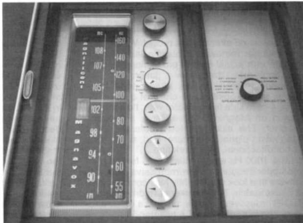
Figure 3. The controls are the typical tuning, power, function, loudness, treble and bass. Also included are a tuning meter and speaker selector offering five main and remote speaker combinations.
