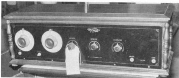
*A Hy-Power Super from Victoreen Radio Company. This 2-dialer superhet has three rheostats to control filament voltages.*
