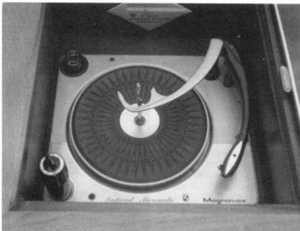
Figure 4. The changer is a British Collaro with an Electro-Voice ceramic cartridge.
