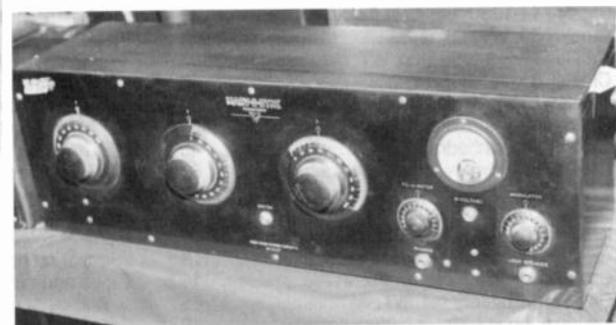
A 3-dialer Marv-O-Dyne Model 612-C by the Amber Manufacturing Co., New York City. This battery-operated set included a meter for monitoring filament voltage.
