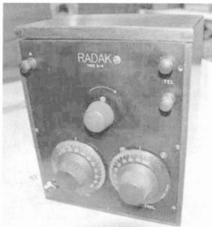
This Clapp-Eastham RADAK R-4 receiver with a 201A tube went for \$170.
