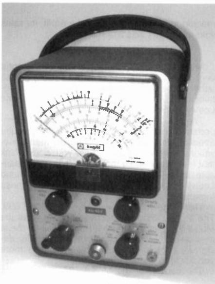
Figure 1: Nearly everyone who reads *A.R.C.* probably built and owned a Knight-Kit VTVM similar to this, or the Heathkit equivalent. Priced at about \$25, they were the foundation of any electronics hobbyist's complement of test equipment.
