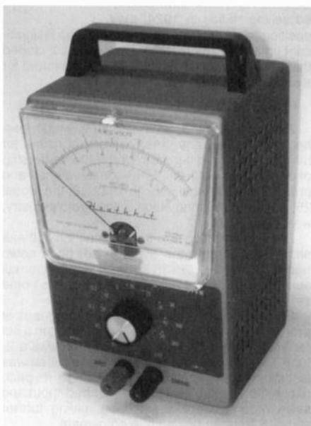
Figure 2: The Heathkit IM-21 AC VTVM and its variants provided ranges covering 10mV to 300V, flat within 1dB± from 10 Hz to 500 kHz. They cost about 20 percent more than the standard VTVM.
