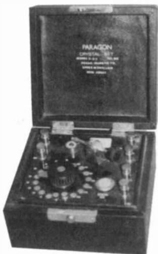
**PARAGON MODEL DX-1** – This crystal set, ca 1924, is housed in a black leatherette case that measures 5 $\frac{3}{4}$ " x 3 $\frac{3}{4}$ ". It has a push button and a buzzer to test the best spot on the galena detector. (Wally Worth – Wollaston, MA)
