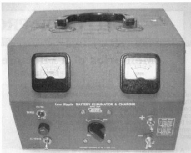
Figure 3: This ratty looking example of an EICO Model 1060 provides 0-8 VDC at 10A continuous or 0-16 VDC at 6A continuous using a transformer with a sliding tap on each of its dual secondaries, and a rectifier with plates the size of a slice of bread. The "Low Ripple" designation on the front panel derives from the Model 1060's extra L-C filter section, not provided in the standard model, the 1050.
